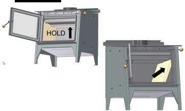
While holding up the baffle assembly horizontally, insert the opposite side brick in from underneath it, as shown above. The 2 side bricks will now support the Baffle.
