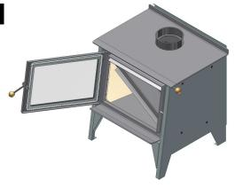
Put the Vermiculite Board baffle brick in first on an angle through the door frame, then repeat for the steel baffle. Join the two parts together & lift it up holding it horizontally resting on the one side bricks.
